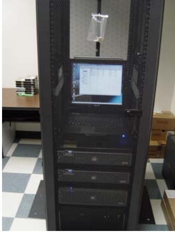
Rack mountable servers save on space and improve airflow.
